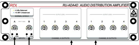
WITH NORMAL INPUT SIGNAL CONNECTED, TRIM INPUT GAINS FOR CORRECT LEVEL ON DUAL-LED METERS (GREEN LED BRIGHT AND RED FLASHING OCCASIONALLY)
