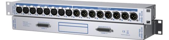
The RME DTOX-16 breakout panels are the perfect rack solutions for interconnecting multichannel XLRs with the common D-sub connector format. Three different versions are available: DTOX-16 I, DTOX-16 O and DTOX-16 I/O. DTOX-16 connects up to 16 XLR inputs or outputs (XLR Neutrik connectors) with two D-sub 25-pin connectors.
