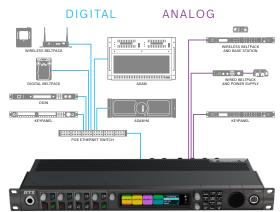
Software upgrades allow for increased capacity and functionality as needs evolve. Users requiring both analog and digital should upgrade to OMS Intermediate or OMS Advanced.
