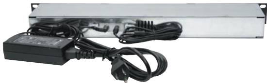
Rear View - 110/220VAC Power Supply
