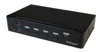
This 4-Port USB 3.0 HDMI® KVM switch lets you control four HDMI computers with a single monitor, keyboard and mouse. The KVM also features 3.5 mm audio and a built-in 3-port USB 3.0 hub.
