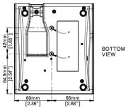
\* Drill blind hole  $\not O$  2.5mm, maximum depth = 6 mm for M3 thread cut.(bottom tap)
