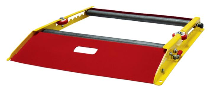
The SMP-RP-27 reel roller system is ideal for storage, dispensing and management solutions of cable reels ranging from 12" to 48" in diameter. The SMP-RP-27 can accommodate cable drums up to 27" wide with weights up to 1,500 pounds. The seven (7) gauge steel frames include six (6) position adjustments for the rollers, a slanted loading ramp, front roller locks for easy loading & unloading, and pre-drilled holes for permanent mounting applications.
