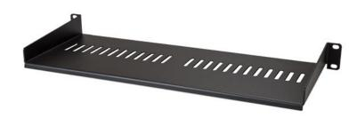
This 1U rack shelf lets you add 7 in. of flat storage space to any EIA-310 compliant server rack or cabinet. The shelf is vented to improve air flow and help lower temperatures in your rack.
