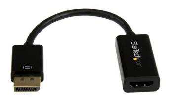
The DP2HD4KS DisplayPort to HDMI adapter enables you to connect a DisplayPort-equipped desktop or laptop computer, such as the HP EliteBook 8570p / 8470p, to an HDMI display. This adapter is compatible with DisplayPort 1.2 & HDMI 4K @ 30 Hz and as a result can support video resolutions up to Ultra HD (4K) as well as the accompanying digital audio up to 7.1 channel surround sound.
