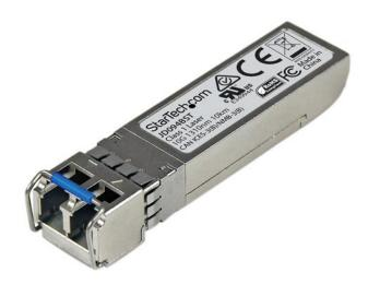
This HP® compatible 10 Gigabit fiber SFP+ is engineered by StarTech.com to deliver what you want most in your network connections: reliable performance. Built to exacting specifications and fully tested to ensure maximum performance, you can install this high-quality fiber transceiver module into HP networking devices that support the HP JD094B transceiver module, as well as other major brands of networking equipment.
