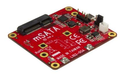
Increase the data storage capacity of your Raspberry Pi or other development board, by connecting it directly to an mSATA drive. Perfect for custom projects and applications, this USB to mSATA converter supports all models of Raspberry Pi as well as other development boards.
