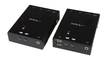
This HDMI extender kit uses HDBaseT 2.0 technology, enabling you to extend 4K HDMI video and four USB 2.0 peripheral devices to a remote location up to 295 feet (90 meters) away, using a single CAT5e or CAT6 cable. The extender can extend 1080p (HD) video even further at up to 330 feet (100 meters).
