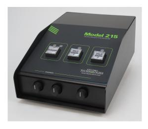
the talkback output channels. These are the audio signals used to communicate with producers, directors, spotters, or other behind-the-scenes production personnel. A status LED is associated with each of the talkback pushbuttons. The pushbutton switches use gold-plated contacts for reliable long-term operation and include backlighting using white LEDs. Three rotary controls allow the user to adjust the content and level of the headphone output.
