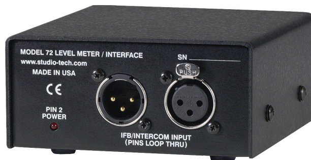
View showing IFB/intercom input and power present LED indicator
