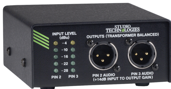
View showing level meters and audio outputs
