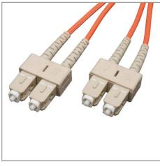
**Description**Tripp Lite's 4 meter ( 13ft ) multimode duplex fiber optic SC/SC patch cable is manufactured from 62.5/125 zipcord fiber. The cable has SC connectors on each end, a PVC jacket and is FDDI and OFNR rated. duplex multimode fiber is most commonly used in LAN applications.
