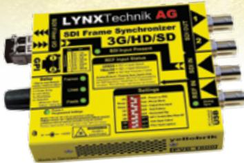
A broadcast quality compact SDI frame synchronizer featuring multiformat support for SDI formats up to 3Gbit/s with optional fiber optic I/O which can be configured to automatically switch between the electrical and optical input if a signal loss is detected. Video processing utilizes robust "flywheel" synchronization that will accommodate a wide variety of low quality asynchronous SDI sources.
