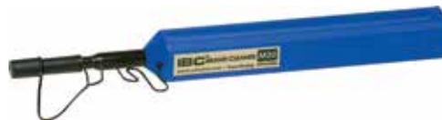
Mechanical cleaning tools designed to clean connectors residing in an adapter or faceplate and unmated connectors. Tools use a novel dry cleaning strand to gently sweep and lift away dust and residues from the connector end face.
