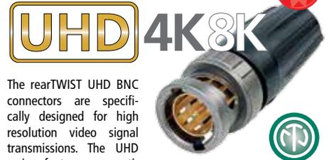
The rearTWIST UHD BNC connectors are specifically designed for high resolution video signal transmissions. The UHD series features an optimized insulator design and reduced crimp diameter from center pin to achieve increased headroom when compared to conventional BNCs. It offers additional return loss reserve for potential impedance deviations resulting from cable bending, incorrect connector assembly or faulty connection interfaces without signal interruption.
