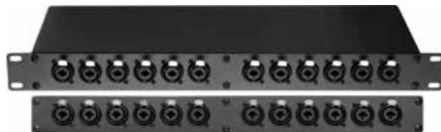
The industry's only XLR-1/4" combo feed-through patch panel! By customer request, we now manufacture XLR-1/4" TRS Combo to XLR-1/4" TRS Combo patch panels. Saves tremendous rackspace! Panel includes 24 (total) high quality Neutrik NCJ6F1-S combo connectors wired in line all housed in a heavy duty 1RU x 6" Deep steel cabinet. Other Configurations available on special order.
