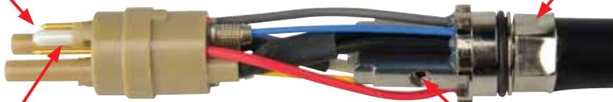
Pins Properly Crimped & Inserted
