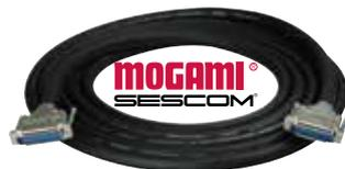
DB25 male to DB25 male with 8 channels analog audio in or out. Cables are crafted with Mogami super flexible 2932 cable. All channels are individually shielded twisted pairs of #26 AWG gauge conductors, with #25 AWG drain. Cables are designed with Industry
