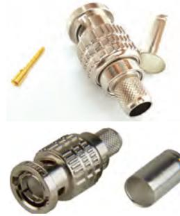
Canare's BCP-D55UHD is their most advanced BNC plug that was developed for use with their 12G-SDI UHD video coax cable the L-5.5CUHD. The return loss at 12 GHz is 15 dB, 26 dB @ 3 GHz and 20 dB @ 6 GHz. The installation work on the cable is a crimp method which enables quick and reliable machining to go along with its Long sleeve shape, insulator locking mechanism, etc.
