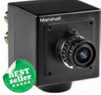
2.5 Megapixel 1/3-inch CMOS Sensor • 3.7mm Megapixel M12 Prime Lens installed (interchangeable) • 1920x1080p 59.94/29.97, 1920x1080i 59.94, 1280x720p 59.94/29.97fps • 3G/HD-SDI (BNC) & CVBS (BNC) built into rear panel • Captures sharp & vivid color images at 0.2 lux (low light sensitive) • WDR function supports high speed & high sensitivity to various light sources
