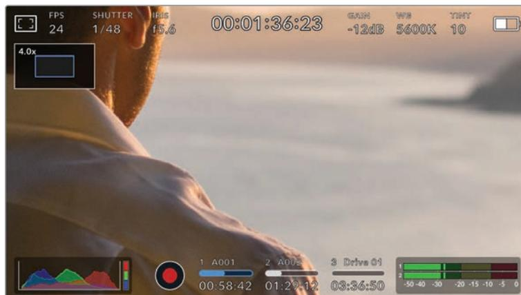
While zoomed in, an indicator in the top left of your LCD touchscreen will show which part of the image you are viewing. You can move around the image using the menu wheel or by dragging your finger around the screen.
