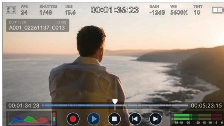
The LCD touchscreen displays a timeline of segments representing all the recorded clips. Each segment in the timeline represents an individual clip. The current clip name and number is shown at the top left of the display and the total number of clips on the card or drive is shown in brackets.
