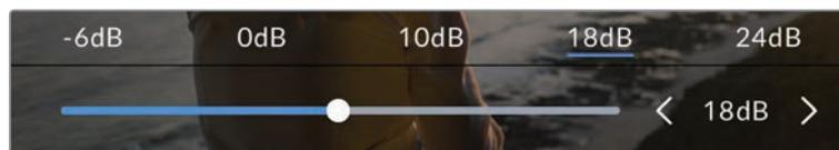
While in the 'gain' menu, your URSA Broadcast G2's gain settings appear along the bottom of the LCD touchscreen. The slider and arrows below the presets let you adjust the gain in 1/3 stop increments.
