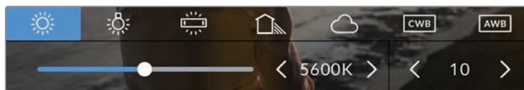
Tapping the white balance and tint indicator on your URSA Broadcast G2 gives you access to five presets, as well as a white balance indicator and slider on the left, and a tint indicator on the right. Adjust these to set a custom white balance for your lighting conditions
