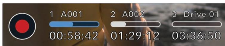
Your URSA Broadcast G2's storage indicator will display the name of your CFast card, SD card, SSD or USB flash disk and the remaining record time
