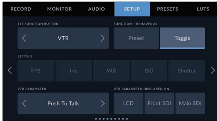
Configuring the 'vtr' button on a B4 lens to function as a 'push to talk' button
